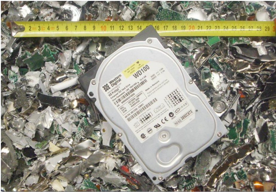
Before and after shredding with JBF HD 15/40 or JBF HD 20/40
