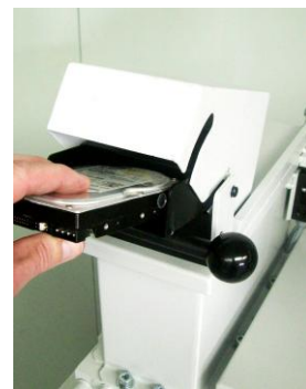
Feeding channel for manual feeding of hard discs
