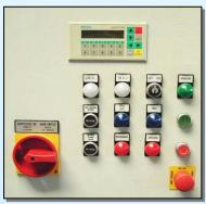
The operation panel at the electrical cabinet contents all relevant operation elements, which allow a reliable operation. The personnel security is assured by security switches on revision openings to prevent against unauthorized access into the cutting zone.
