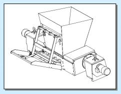
Inside the feeding funnel a mechanical, electromotive or hydraulic driven pushing device can be installed to enable a continuous operation even with problematic-to-handle cutting material.
