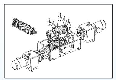
Enabling the lift-out of the entire cutting shafts, the divided frame of the cutting unit allows a fast exchange of the cutting unit, if requested.
