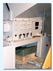
An accurate classing of the cutting material can be enabled by installing a granulate screen underneath the cutting unit. The screen hole size will be adapted to the according request.
