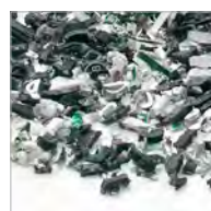
Particles of shredded USB sticks. Cutting size 20 x 40-50 (<1000 m²).
