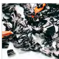
Particles of shredded magnetic tapes, credit cards and customer cards. Cutting size: 20 x 40-50 (<1000 m²).
