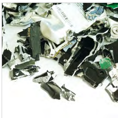
Particles of shredded hard drives Cutting size: 40 mm. Security level: H-3
