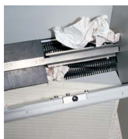
Automatic mechanical feeding system with revolving flaps
