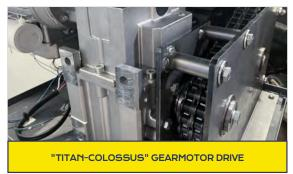
The Kobra GAMBLER is eqipped with the "Titan-Colossus" gearmotor drive specially designed heavy duty cutting knives with unmatched power to shred large quantities of casino gaming pieces such as dice, chips, gaming tokens and playing cards.
