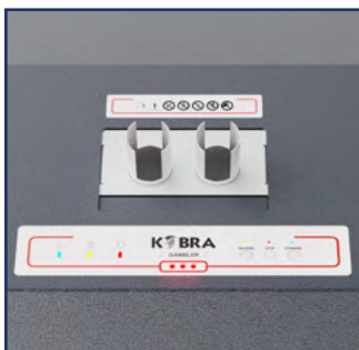
Special feeder with two openings for automatic destruction of up to 2000 fiches per hour.
