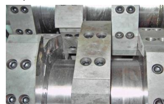
Segment knives, can be exchanged without dismantling of the cutting shafts
