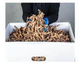
Making cardboard chips for packaging and filling material. The cardboard chips stabilize the goods in the package, fill up empty spaces and cushion impacts - and all that without plastic.
