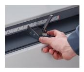
Depending on the application, the cushioning volume of the packaging material can be adjusted as required.
