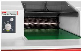
The material feeding is convenient and takes place via the non-slip conveyor belt.
