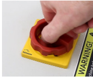
Turn isolator on
