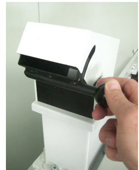
Feeding channel for manual feeding of hard discs
