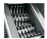
The induction-hardened, solid steel cutting rollers are robust and ensure a high level of durability!
